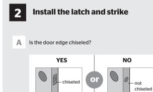
Use latch "A". If the Use latch "B" (not latch bolt is not already extended, extend the latch bolt as shown. extended, extend the latch bolt as shown.
